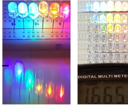
Figure 1.3: A light emitting diode, LED, has a specific colour.
